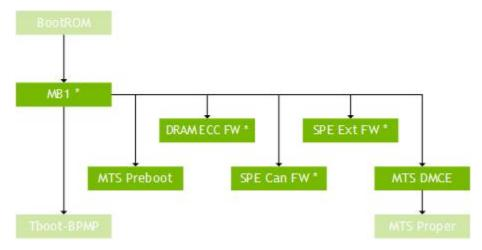
• **MB1**: Loads MTS Preboot and verifies it using the double verification mechanism. It first verifies the OEM credential, then the NVIDA credential (using MAK/MDK).
