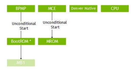
• **BootROM**: Loads BRBCT and establishes a trusted OEM public key by computing the hash and comparing it to the fuse settings. It then verifies the BCT using the OEM authority (i.e. the public key).
