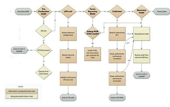
If authentication fails, the Boot ROM automatically goes into USB Recovery mode and waits for input via the USB. The Boot ROM never yields control from Recovery Mode except to authenticated code or error messages.
