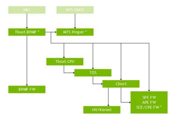
**TBoot-BPMP**: This is the main binary loader in the boot flow. It loads the binaries that are required to start CPU execution. These binaries are owned by the OEM, and are verified and decrypted using the OEM authority.
